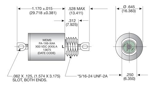
Tolerance:  $\pm$  .010 ( $\pm$ .254 mm) unless otherwise specified. \*All units supplied with internal tooth lockwasher and hex nut. For further details see page 6.
